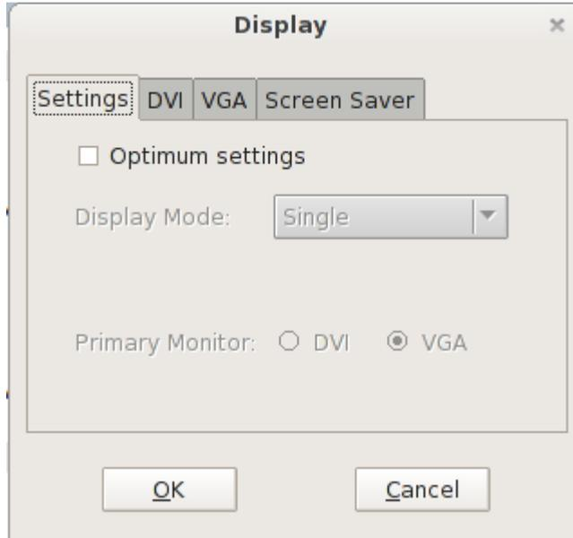
When one monitor is connected, Display Mode is “Single”, the option is grey and unselected.
